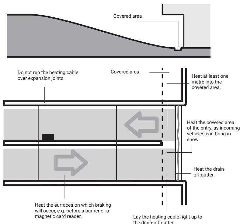
First make sure that the area to be heated complies with the data in the design instructions. Establish where the junction boxes are to be installed and check that the connection leads are long enough.
