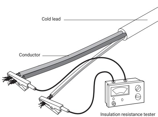
The insulation resistance should be measured with the aid of a 2500 Vdc (500 Vdc minimum) insulation resistance tester. The reading should be more than 100 MΩ. Record all the measured values on the Installation Test Record provided.
