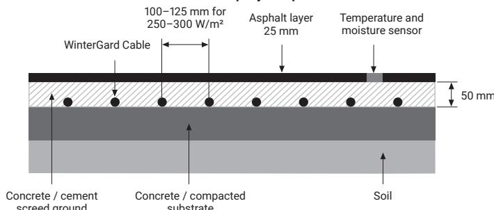
If the heating cable can not be fixed to a reinforcement mesh, the installer should use the plastic spacer (for asphalt metal VIA-SPACER) or other fixing method to keep the cable spacing consistent.
